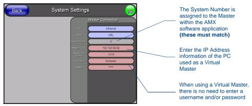
FIG. 30 Sample System Settings page (for Virtual Master communication)
